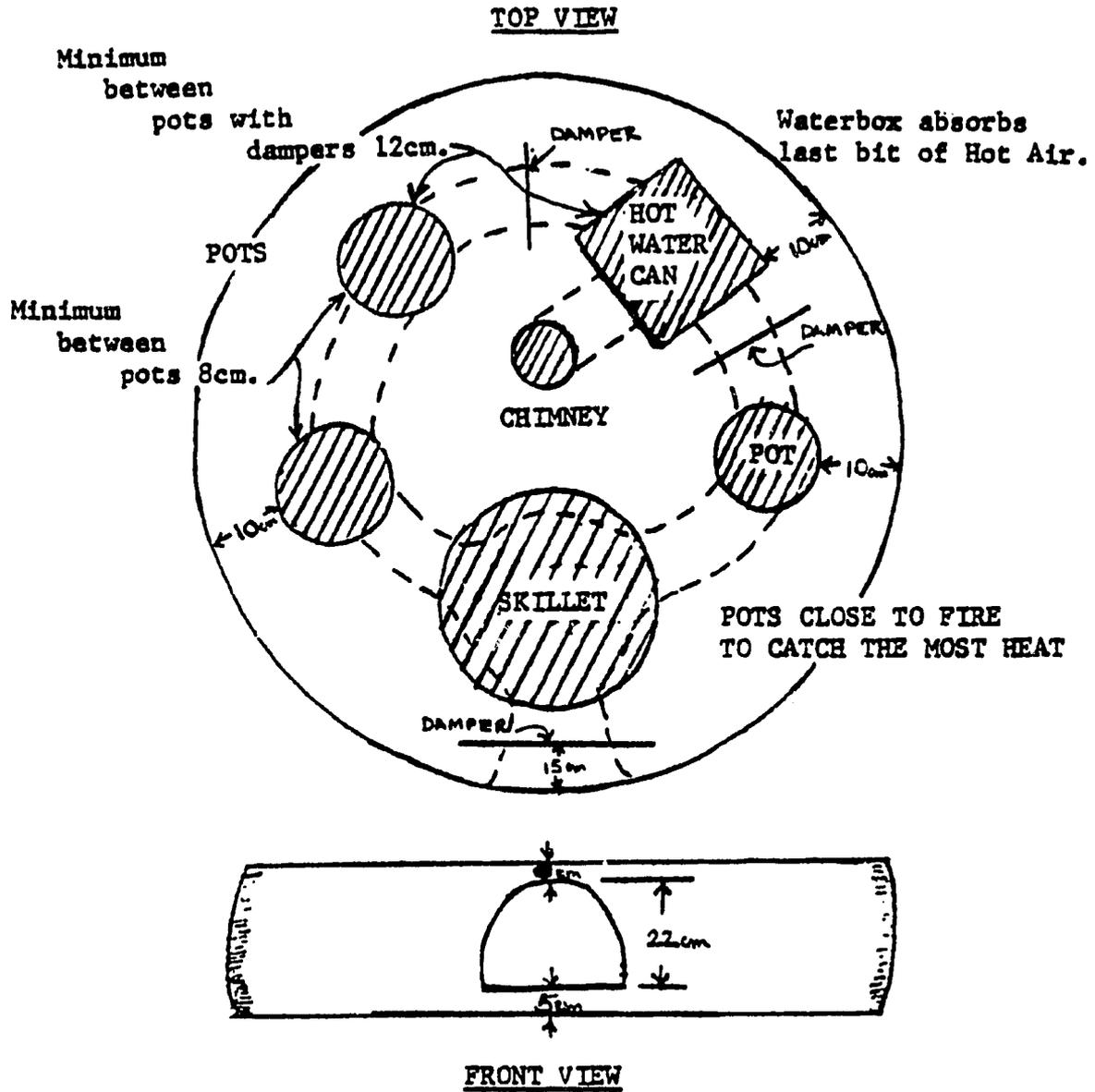
Locate the firebox at the front center of the stove. Arrange pots so that they are closest to the heat source. Diagrams show the positions of hot air tunnels and dampers; a cooking hole located near the chimney provides enough heat to keep water warm for washing.
