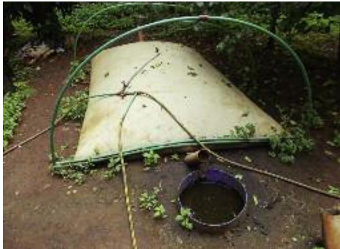
As microbes digest the organic material, biogas bubbles up from the mixture, inflating the plastic bag. Sitting above the ground in the sun, the system quickly heats up, promoting rapid production of methane gas. It is then piped through a PVC tube connected to an appliance or piece of equipment such as a gas stove for cooking.
